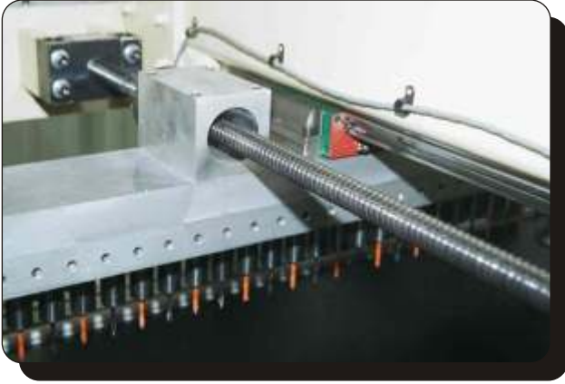
R75 Drill Row Ball Screw and Linear Rail Positioning Provides for Precision Drill Row Location.
