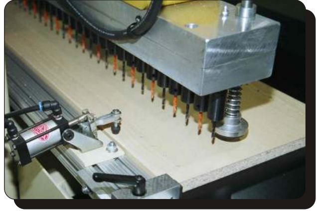
R75 Material Clamping and Back Fence Positioning Allows for Accurate Drilled Hole Locations.
