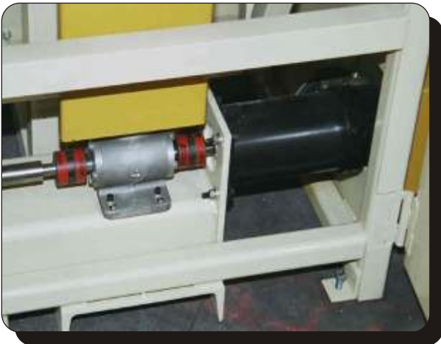
R75/R150 Servo Driven Triple Ball Screw Table Feed Control Allows for Precision Drill Depth Control and Through Feed Boring.
